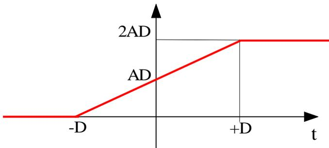
$$z(t) = \begin{cases} 0 & t < -D \\ A(t + D) & -D < t < +D \\ 2AD & t > +D \end{cases}$$
